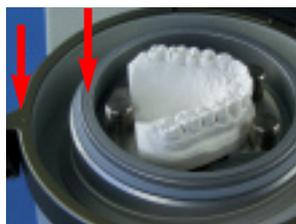
2. Put the model pot into the Erkoform-RVE unit, the markings (arrows) have to be opposite.
