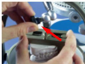
6. Close the hydraulic joint in this position.
