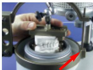
4. When the supporting pin is contact, the models can be put into occlusion, with or without a construction bite.
