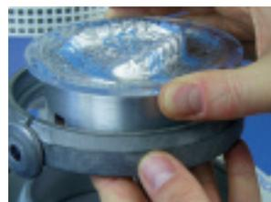
**14 b.** ...and remove the model. Therefore lift the foil holder of the Erkoflex-RVE, hold the model pot from below, release the frame ring and take off the model with the model pot.
