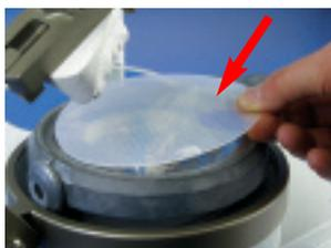
**2.** Quickly close the Occluform except of about 1 mm. Open the Occluform again, remove the foil Erkolen and...
