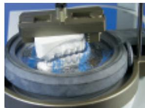
**12 b.** Fill up with granules, thermoform - here Erkodur 4 mm - and immediately close the Occluform until the supporting pin is in contact.
