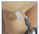
**4.** Round off and smooth cut edges with the abrasive stone without damaging the plastic coating.
