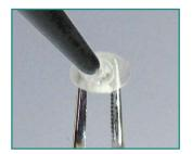
4. Then immediately put on and hold with light pressure until the adhesive gel is well dispensed under the hook. Do not let slip while the adhesive is drying.
