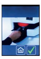
to 6 + 7. After the cooling time the display shows the further steps to pull the model pot out of the unit and remove model and foil out of the foil reception (q - i).
