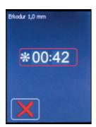
**to 5.** After thermoforming the cooling time runs backwards.
