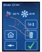
**Recommendation:** If an Erkodent foil will be saved with the factory parameters and as a favourite with changed parameters, the changed one should be saved as new foil with a different name in order to avoid any mix-up.
