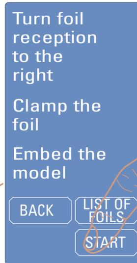
to 2. Swivel foil reception upwards and then to the right (a). Take out foil securing ring, put in the selected foil Erkodur 1.0 mm and clamp with the foil securing ring (b). Embed the model now or during the heating process in the granules. (c). Please choose "start".
