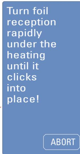
to 3. For better clicking into place slightly push the grip cavity downwards. When it clicks in, the heating switches on (d + e). The functional field "abort" stops the standby mode or the heating process and leads back to display 2. If the foil is turned out of the heating contact, this display is shown as well.
