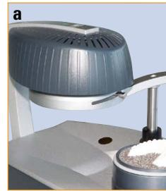
**Note**, switch on the vacuum pump only with the foil reception in the upper position.
