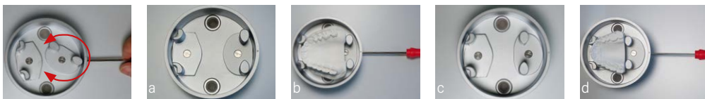
Model pot: turnable clamping plate, position for the most models (a + b) and for small models (c + d).
