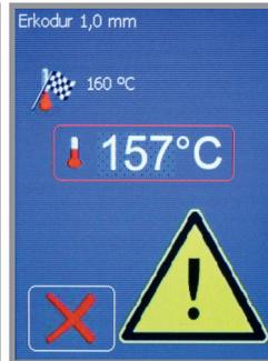
**to 3.** 10 °C before reaching the rated temperature, a signal sounds and a warning sign flashes. As soon as the rating temperature is reached, the thermoforming process will be automatically released.
