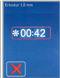
**to 4.** After thermoforming the cooling time runs. Afterwards further working steps are indicated on the display.
