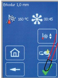
**to 1.** Correct foil?, if yes, confirm. In the display further working steps are indicated. The visualisation disappears with the next step. If necessary, move support for foil frame in the upper position.
