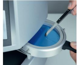
To determine the cooling time, stop the time from beginning of the adaptation. For the first time after approx. 1 minute select cooling time »STOP«, the cylinder moves upwards, the foil can be pulled out. Manually check the foil temperature, **attention risk of burning!** The right cooling time is achieved if the foil has approx. room temperature on the surface. The foil can now be saved as described under "enter new foils".
