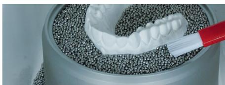
Remove granules with the supplied magnet. **Never clean by blowing out!**
