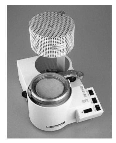
Vacuum thermoforming unit for the dental thermoforming technique. With electronically controlled working procedure. Independent on compressed air. With integral vacuum pump and vacuum reservoir (patented).
